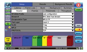
Automated tests compliant with RFC2544 with configurable threshold values and maximum transmit bandwidth settings Throughput, Latency, Frame Loss, and Back-to-Back (burst) tests
